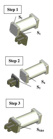
Fig. 9: Assembly operations for CAD parts
